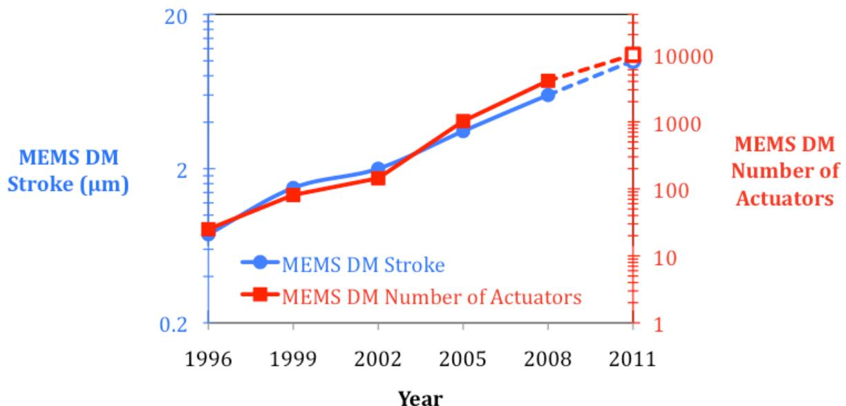
Figure 2: A history of DM peak achievable stroke and actuator count for the MEMS DMs pioneered at BU. Data correspond to fully functional deformable mirror devices with >99% working actuators (100% for devices with 1024 or fewer actuators) and optical surface quality. Results for 2011 are projected.
