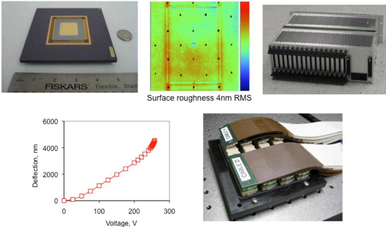
Figure 3: Engineering grade 4092 actuator MEMS DM. Clockwise from top left: Photo of the DM in its package; interferometrically measured small scale surface flatness ~4nm rms; Electronics driver; Back side of package, with eight 512-wire ribbon cables; Measured voltage vs. deflection curve.
